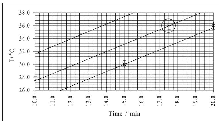
Here we see that the deviations of the points from the best line are much larger than the error bars. What if John really found such large deviations? He would suspect that something must be wrong with his experimental method to produce such large temperature fluctuations. Perhaps he sometimes forgot to stir the water, so that it was not always at a uniform temperature when he read the thermometer.
