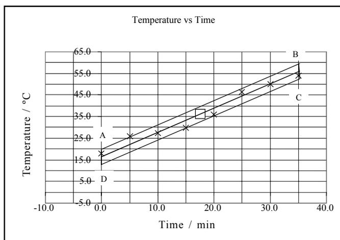
As the points are all of equal accuracy (reading uncertainties in  $t$  and  $T$  being the same for all readings) then it can be shown that the best straight line through them passes through their **centroid**. This is the 'centre of mass' of the points; its co-ordinates are the means of all the  $x$  and  $y$  values. Here the centroid is the point (17.5, 36.0) and is marked with a square.
