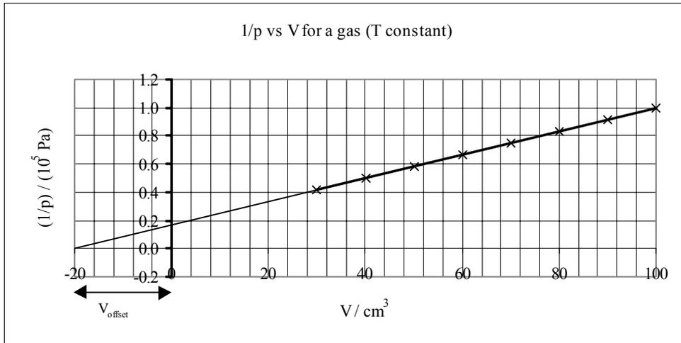
This shows clearly the offset in the volume, which is identified with a dead-space in the equipment. In this case there was a dead-space of  $20 \text{ cm}^3$ . The apparatus may be redesigned to reduce or eliminate this. The results can be corrected to allow for the dead-space, and the linear relationship can be shown to hold:
