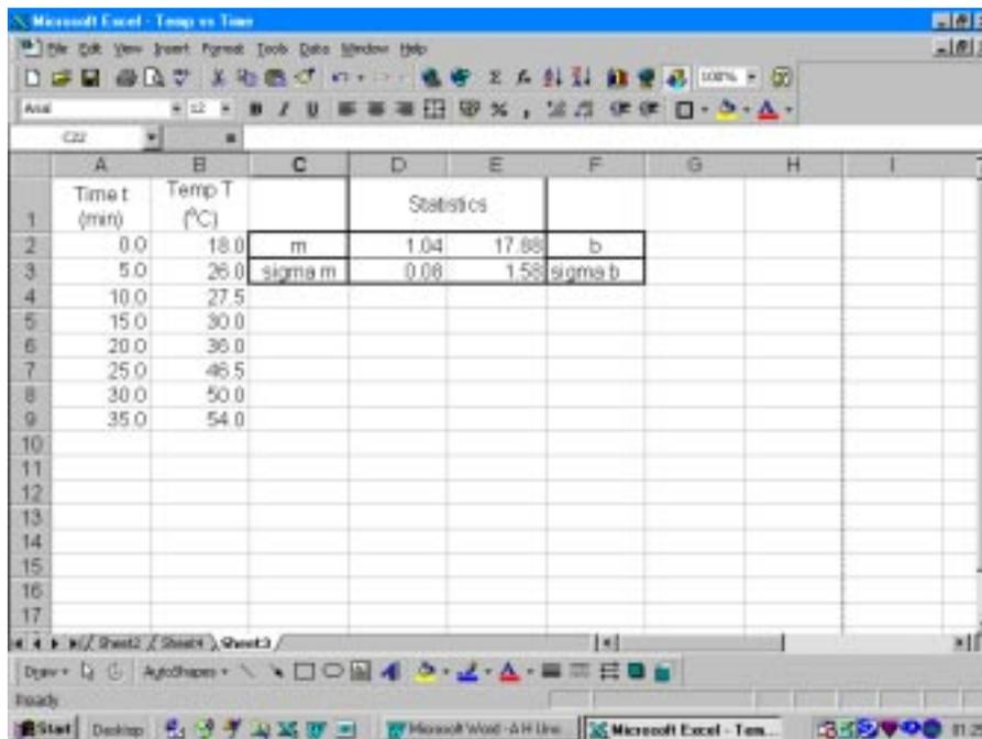
The top left cell which you highlighted contains  $m$ , and the top right cell contains  $b$ . The standard deviation of each is the box immediately below it.
