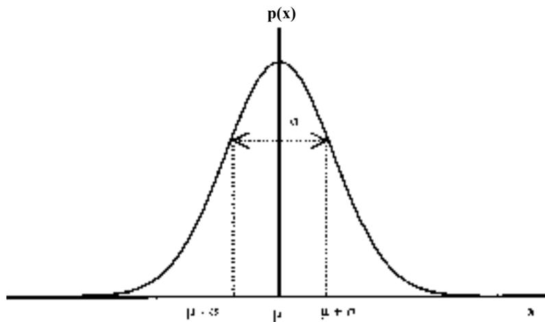
Figure 10 shows a graph of the normal distribution curve, in which  $p(x)$ , the probability of obtaining a value  $x$ , is plotted against  $x$ . The curve peaks at  $x = \mu$ , the mean value, which is (in the absence of systematic effects) the true value of the quantity being measured. The equation of the curve is:
