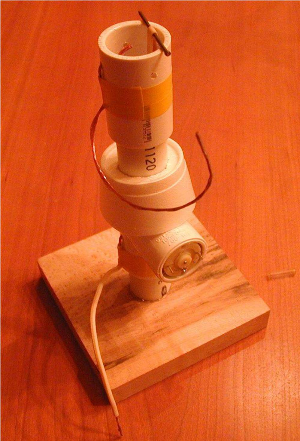
We need a small glass tube to act as both a low-friction top pulley, and as a "triboelectric" complement to the rubber band, to generate static electricity by rubbing. Glass is one of the best materials to rub against rubber to create electricity.
