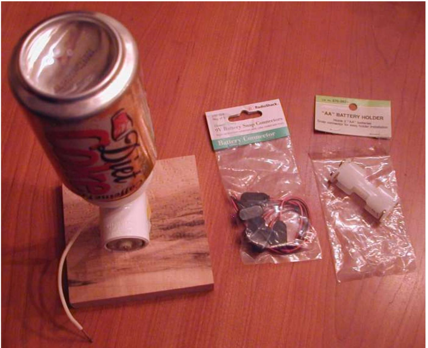
To use the Van de Graaff generator, simply clip the battery to the battery clip. If the brushes are very close to the ends of the rubber band, but not touching, you should be able to feel a spark from the soda can if you bring your finger close enough. It helps to hold onto the free end of the bottom brush with the other hand while doing this.
