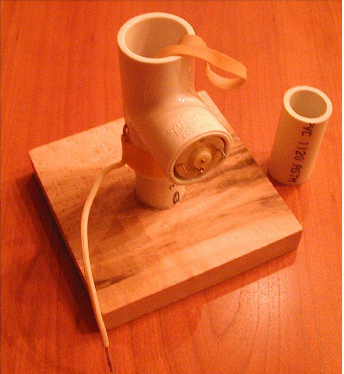
Next, cut another 3 or 4 inch piece of 3/4 inch PVC plumbing pipe. This will go into the top of the "T" connector, with the rubber band going up through it. Use the small nail to hold the rubber band in place, as in the photo below. The length of the PVC pipe should be just enough to fit the rubber band. The rubber band should not be stretched too tightly, since the resulting friction would prevent the motor from turning properly, and increase wear on the parts.
