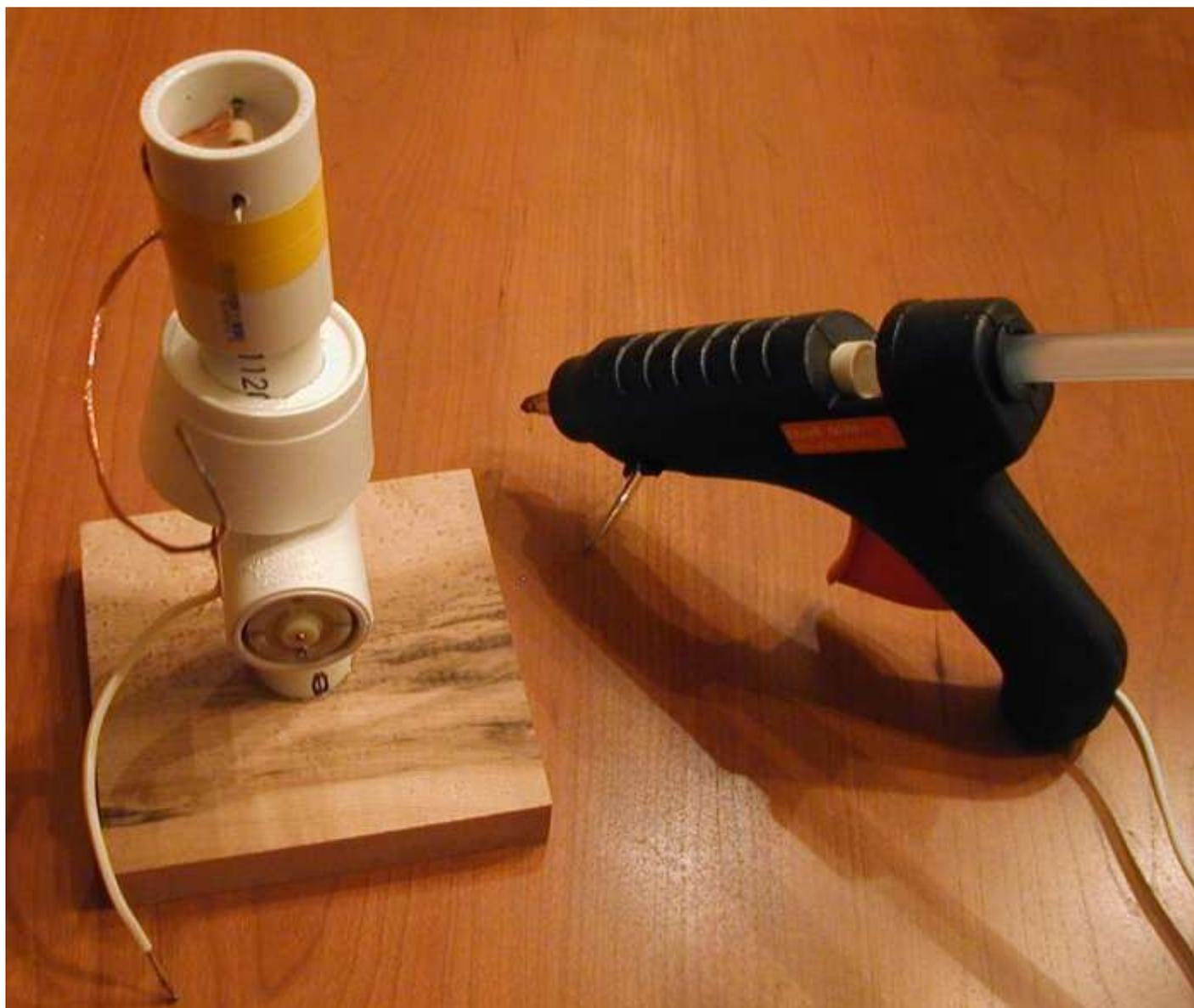
At this point we are ready for the empty soda can. Aluminum pop-top cans are good for high voltage because they have nice rounded edges, which minimizes "corona discharge".
