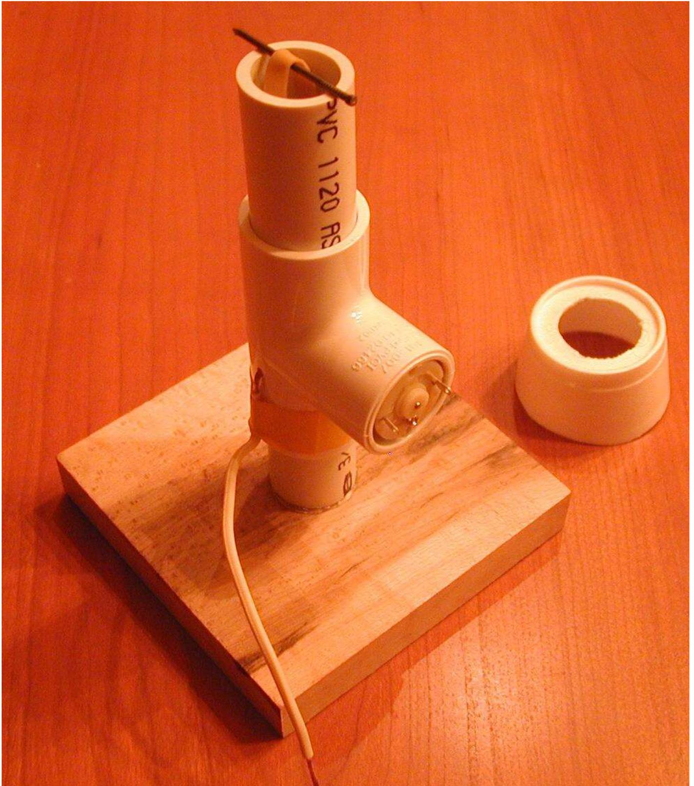
Cut the polystyrene cup about an inch from the bottom, and carefully cut a 3/4 inch diameter hole in the centre of the bottom of the cup. This hole should fit snugly onto the 3/4 inch PVC pipe.
