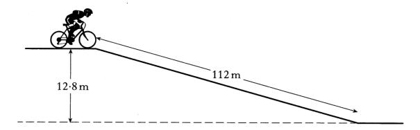
(i) Calculate how much potential energy has been gained by the cyclist and the bike at the top of the hill.
