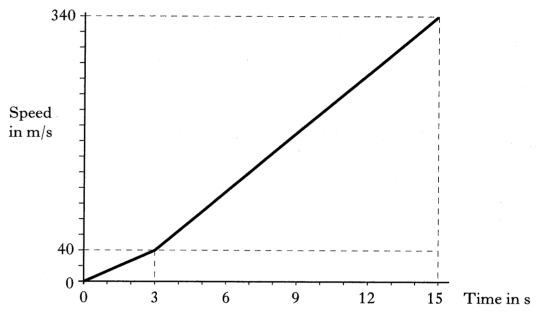
(a) Calculate how far the car travelled during the 15 s shown.
