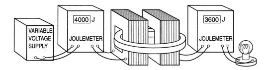
Initially, the displays on both joulemeters are set to zero. The supply is switched on and after a certain time the readings shown are obtained.
