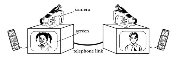
A videophone is a special telephone which can be used to send both video signals (for pictures) and audio signals (for sound) along a telephone link.
