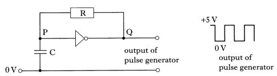
Complete the table to show the voltage at P and at Q when the capacitor in the pulse generator is charged and when it is uncharged.
