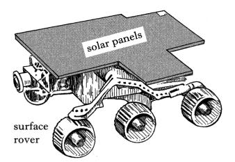
In July 1997 Mars Pathfinder landed on the surface of the planet. Pathfinder consisted of a stationary lander and a mobile surface rover. The lander was in constant communication with Earth and there was a UHF radio communications link between the lander and the surface rover.
