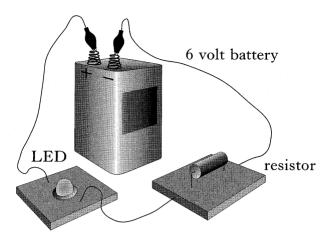
The light emitting diode (LED) is rated at 2 volts and lights at normal brightness.
