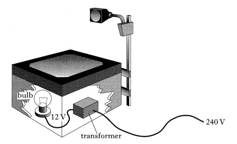
The transformer has 1000 turns in its primary coil. Calculate the number of turns in its secondary coil.
