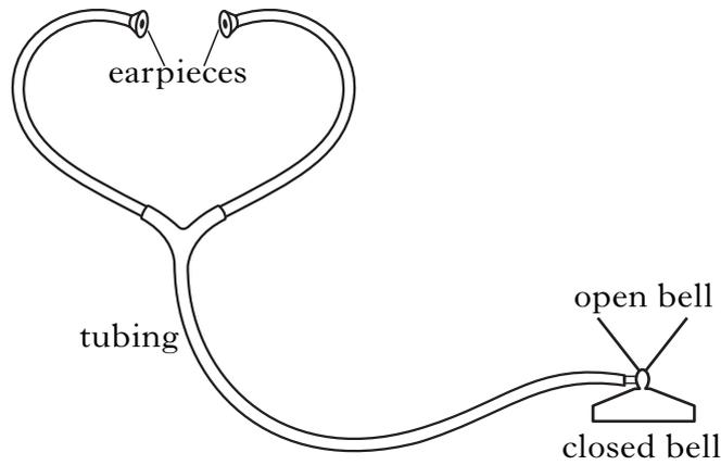
The open or closed bell is placed on the body to detect sounds.
