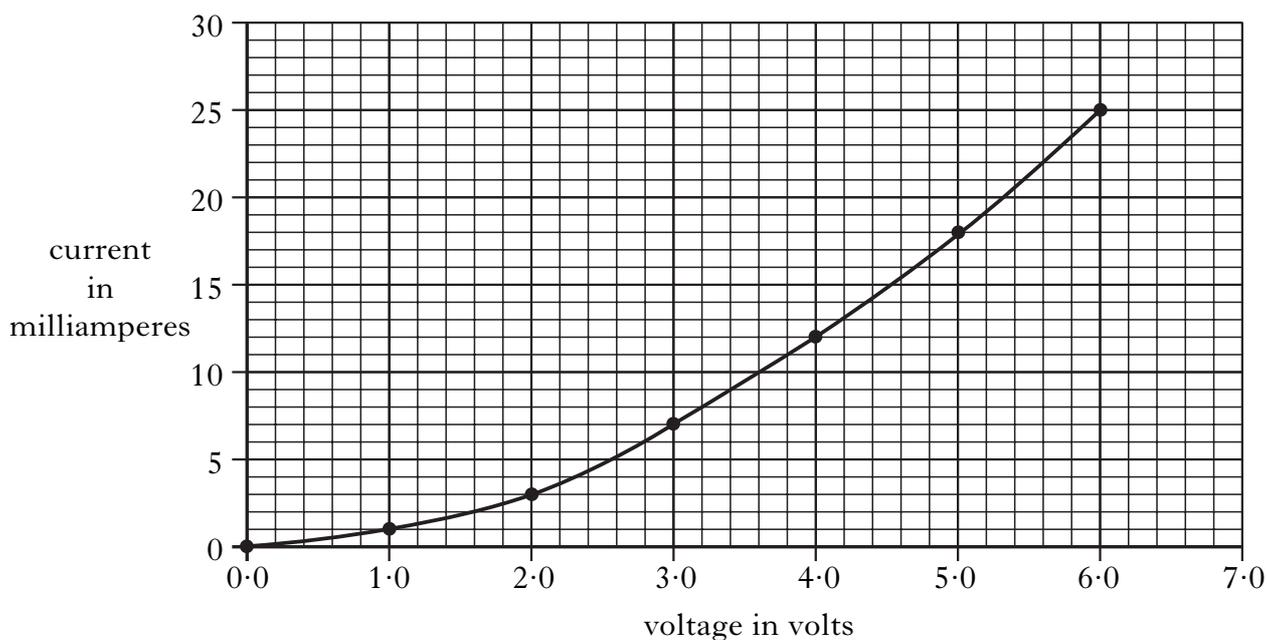
(i) What is the current in the thermistor when the voltage across the thermistor is 5.0 volts?
