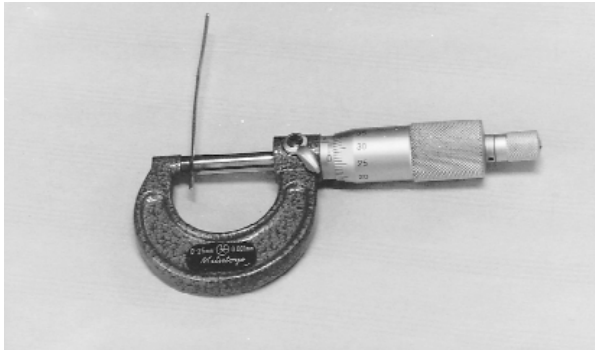
Fig. 3.23 Measuring diameter of wire
