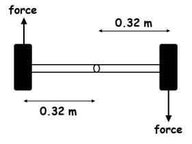
A display firework consists of a 0.64 m long rod of negligible mass, pivoted about its centre. At both ends of the rod, a firework of mass 0.50 kg is attached. Both fireworks are lit at the same time and each provides a tangential force of 25 N perpendicular to the rod, causing the rod to rotate about its central pivot point.
