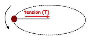
The only force acting in the horizontal direction is the **tension** in the string, so the **tension** must provide the **centripetal force**:
