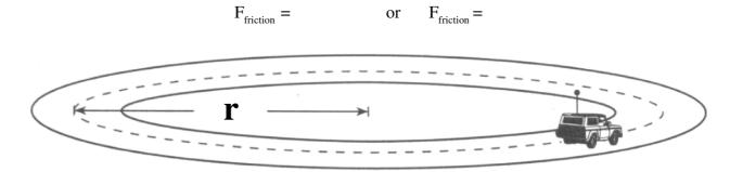
If the vehicle's speed increases to a certain value, the force of friction will no longer be large enough to maintain the circular path - so the vehicle will skid off at a tangent to the curve.
