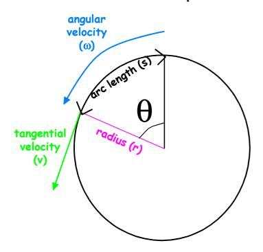
• Carry out calculations involving the relationship between tangential velocity (v), radius (r) and angular velocity (ω).
