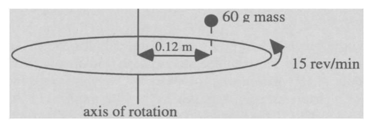
A CD rotates around a central axis at 15 revolutions per minute. The moment of inertia for the CD is  $1.74 \times 10^{-3} \text{ kg m}^2$ .
