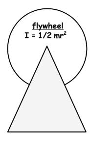
A flywheel of mass 30 kg an radius 0.20 m is mounted on friction-free bearings. A constant tangential force of 20 N is applied to the flywheel by an electric motor.
