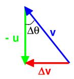
Change in velocity ( $\Delta v$ ) and therefore <u>acceleration</u> are directed towards the **centre of rotation**.
