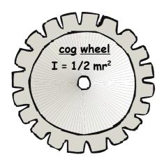
A cog wheel of mass 2.50 kg and radius 0.100 m is mounted on a friction-free shaft.
