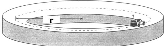
A vehicle is able to travel faster on a banked curve than on a horizontal curve before skidding off at a tangent because the centripetal force is greater on the banked curve - It is provided by a component of the friction force (F<sub>friction</sub>) between the vehicle tyres and road + a component of the normal reaction force (R) of the road on the vehicle.
