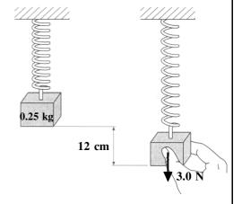
• State and explain this equation for simple harmonic motion:  $d^2y/dt^2 = -\omega^2 y$ .
