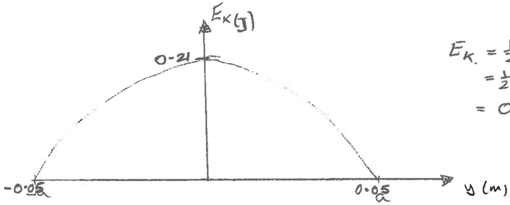
$$\begin{aligned} E_k &= \frac{1}{2} m \omega^2 a^2 \\ &= \frac{1}{2} \times 0.5 \times (10.5)^2 (0.05) \\ &= 0.21 \text{ J} \end{aligned}$$
