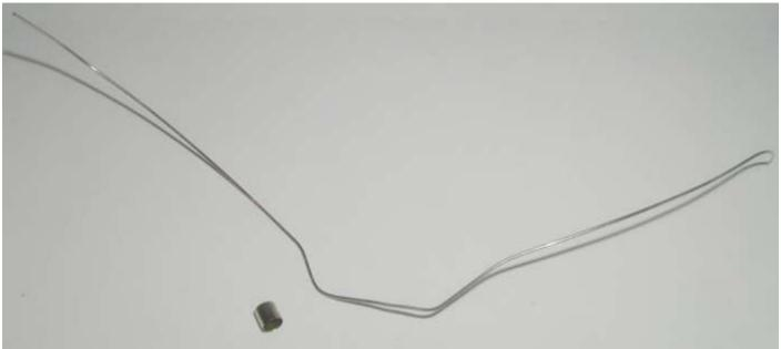
The armature (the part that spins) is made from the other piece of wire and the metal cap we saved when we took apart the fuse. Sharpen both ends of the wire by cutting the ends at a diagonal, like we did with the base wire. Bend the wire into an S shape. The pointed ends of the wire should point at 90 degrees from the centre straight part of the wire.
