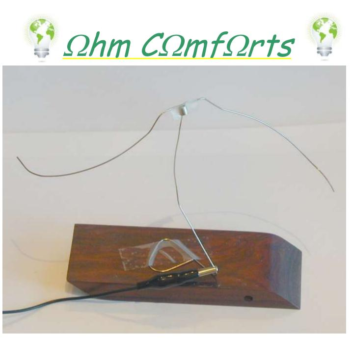
First, take one piece of wire (a straightened paper clip will do), and cut the end at an angle so it is sharp. Bend the other end into a rough loop or triangle, so the wire will stand up with the sharp point facing straight up. A little tape will help hold it onto the table, or a block of wood.
