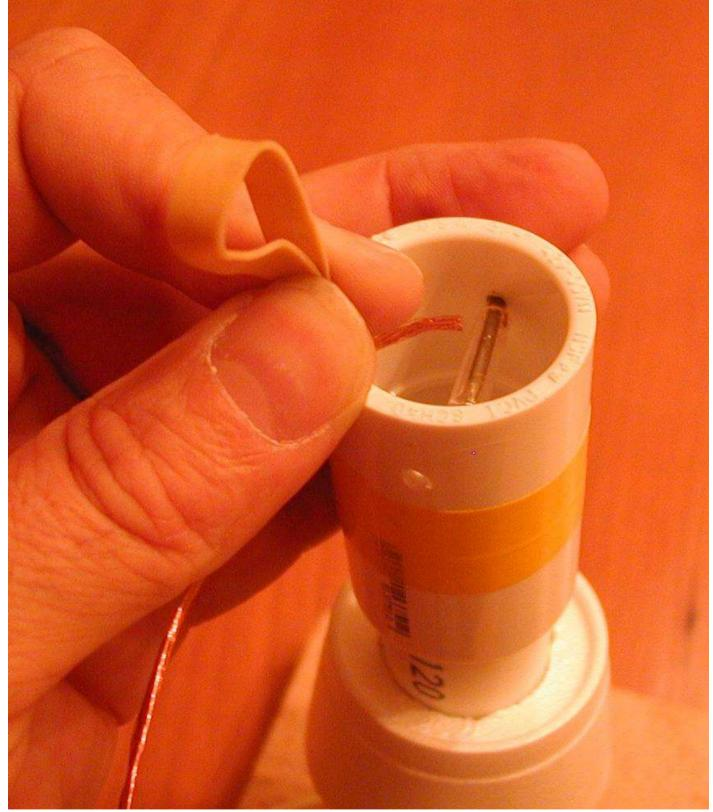
Now we glue the polystyrene collar in place on the PVC pipe. I like to use a hot glue gun for this, since the glue can be laid on thickly to stabilize the collar, and it sets quickly and does not dissolve the polystyrene.
