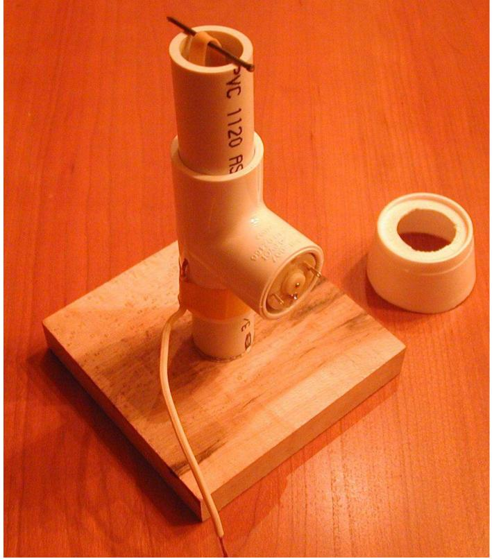
Cut the polystyrene cup about an inch from the bottom, and carefully cut a 3/4 inch diameter hole in the centre of the bottom of the cup. This hole should fit snugly onto the 3/4 inch PVC pipe.
