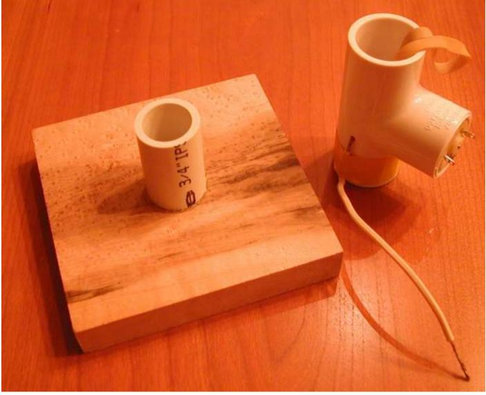
The first thing to do is to cut a 2 to 3 inch long piece of 3/4 inch PVC pipe, and glue that to the wooden base. This piece will hold the generator up, and allow us to remove it to more easily replace the rubber band, or make adjustments.
