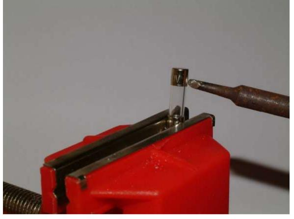
The resulting glass tube has nice straight, even edges, which are "fire polished" for you, so there is no sharp glass, and no uneven edges to catch on the PVC and break the glass.
