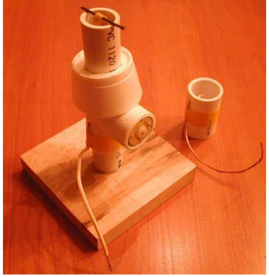
Now drill three holes near the top of the PVC union coupling. Two of these holes need to be diametrically opposite one another, since they will hold the small nail which will act as an axle for the rubber band. The third hole is between the other two, and it will hold the top "brush", which, like the bottom brush, will almost touch the rubber band.
