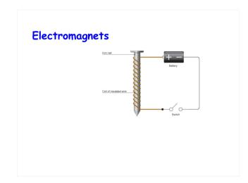
An electromagnet is a magnet that needs an electric current to work
