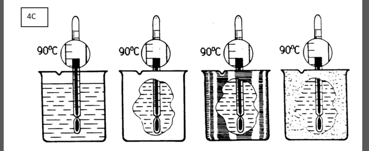
A pupil sets up the following experiment to find out how well different materials keep in heat.
