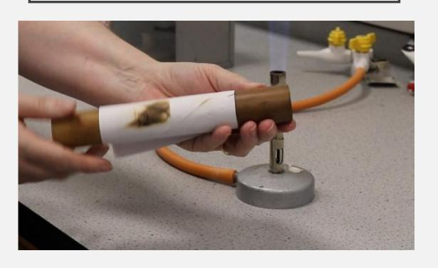
The paper over the wood burns as the wood is an insulator and the heat cannot escape. The temperature increases above the temperature at which paper catches fire.
