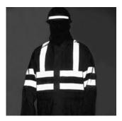
One type of retroflective material is made from small glass spheres partially embedded in a silver-coloured surface that reflects light.
