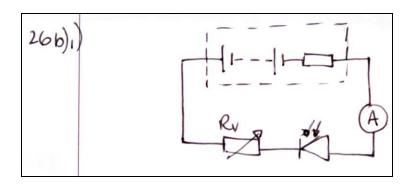
Comment: This candidate has confused the symbol for an LED with that for a photodiode. The polarity is also wrong for it to be forward biased.
