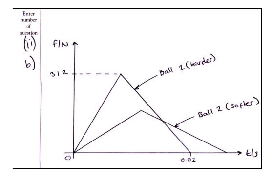
Comment: For part (a)(ii), the graph for the harder material shows a wrong value for the peak force. The time value of 0.02 s is correctly positioned.
