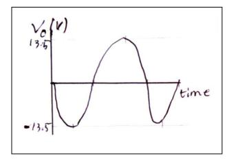
Comment: This candidate has realised that the signal is inverted and that the op-amp saturates. However, the very high gain of the circuit means that even the smallest value of input signal will produce an output voltage at  $\pm 15$  V (approximately). This means that the shape of the output signal should be 'square'.
