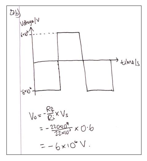
Comment: This candidate has realised that the signal is inverted and that the output is 'square' in shape. However, they have stated that the maximum value is  $\pm 6 \times 10^6$  volts, rather than ±15 V.
