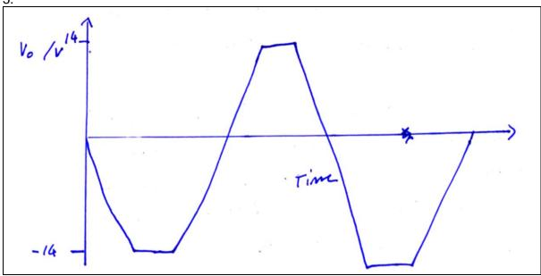
Comment: This answer correctly shows inversion and that the maximum output voltage is near to the value of the supply voltage (ie ±15 V). However, it has not been realised that with such a high gain even the smallest value of input voltage will be so greatly amplified that it produces an output voltage at ±15 V (ie a 'square' wave output).
