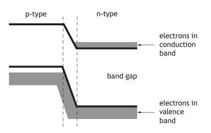
LEDs emit light when electrons fall from the conduction band into the valence band of the p-type semiconductor.
