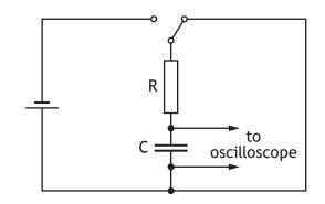
Which pair of graphs shows how the potential difference V across the capacitor varies with time t during charging and discharging?
