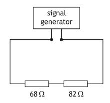
Determine the r.m.s. voltage across the 82  $\Omega$  resistor. Space for working and answer
