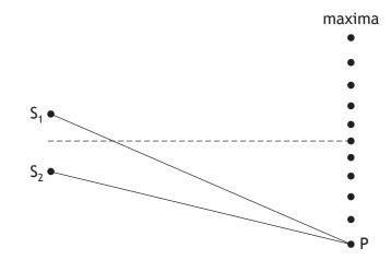
The path difference  $S_1P-S_2P$  is 154 mm.
