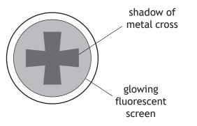
The potential difference between the anode and the cathode is now increased to 2.2 kV. This changes what is observed on the screen.
