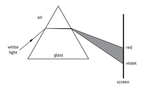
The prism is now replaced with another prism made from a different type of glass with a lower refractive index.
