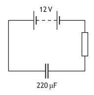
When the capacitor is fully charged the energy stored in the capacitor is
