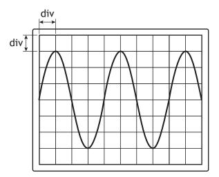
The Y-gain setting on the oscilloscope is 1.0 V/div. The timebase setting on the oscilloscope is 0.5 s/div.
