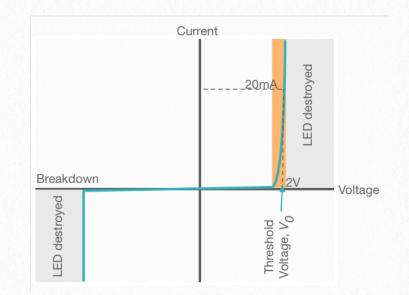
At the threshold voltage,  $V_0$ , LEDs emit photons of energy:
