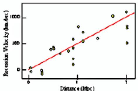
The graph plots the data collected by Hubble giving the relationship between the velocity of a galaxy (recessional velocity) and its distance from us
