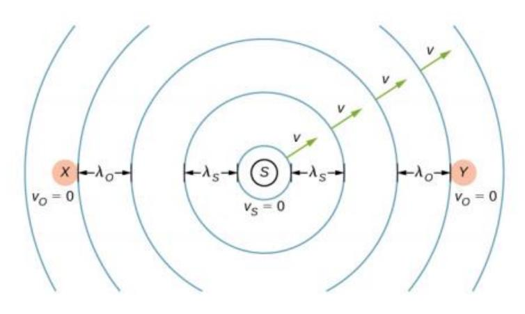
A stationary source sends out sound waves at a constant frequency fs, with a constant wavelength  $\lambda s$ , at the speed of sound v. Two stationary observers X and Y, on either side of the source, observe a frequency fo = fs, with a wavelength  $\lambda o = \lambda s$ .
