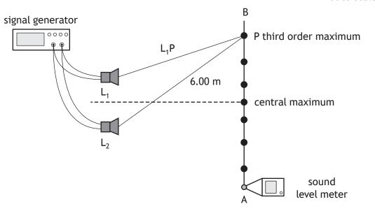
A sound level meter is moved from A to B, and a series of maxima are detected.
