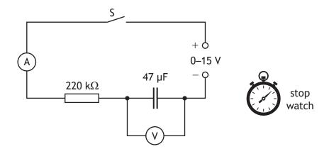
(a) Describe how the results of this experiment are obtained and used to show how the voltage across the capacitor varies with time while the capacitor is charging.
