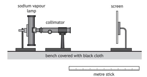
(a) The parallel beam is shone onto a screen. The distance between the end of the collimator and the screen is 0.40 m.
