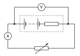
The resistance of the variable resistor is altered and readings of voltage V and current I are taken. These readings are used to produce the following graph.
