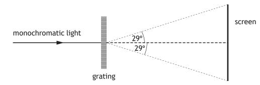
The angle between the central maximum and the maximum observed at the edge of the screen is 29°.
