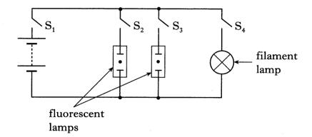
Each of the three lamps is marked 12 volts, 9 watts.
